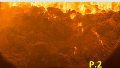
temperature around 1000 degrees centigrade to ensure all dangerous material and gases are totally incinerated. The furnace is on a slope and the material is encouraged down the slope by a series of flaps which activate automatically to
